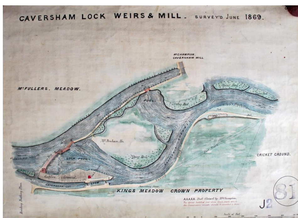
One item from the vast Thames Conservancy archive: a survey of the lock and weirs at Caversham, 1869
